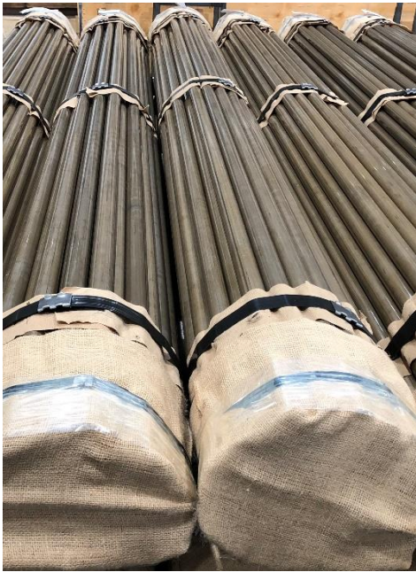
Dark and uniform surface appearance of ASBW hot stamping rod
